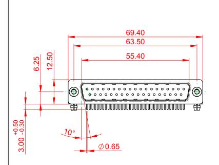
**ISSUE NUMBER** THIS IS A C.A.D. GENERATED DRAWING TOLERANCE UNLESS OTHERWISE SPECIFIED ORIGINAL DO NOT MAKE MANUAL REVISIONS TO MASTER. .X ±0.25 .XX ±0.13 .XXX ±0.10 11.0 ±0.3 6.10
