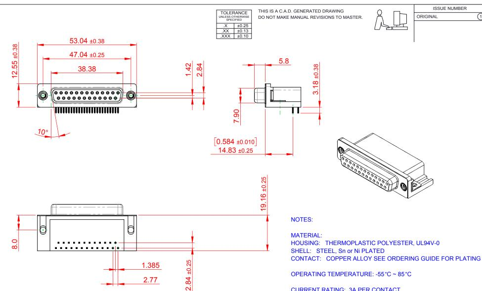
**CURRENT RATING: 3A PER CONTACT** CONTACT RESISTANCE: 25mΩ MAX. INSULATOR RESISTANCE:  $5000M\Omega$  min. **DIELECTRIC**
