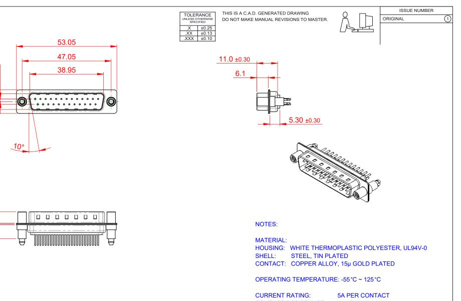
CONTACT RESISTANCE:  $25m\Omega$  MAX. INSULATOR RESISTANCE: 5000MΩ min. DIELECTRIC WITHSTANDING VOLTAGE: 1000V AC rms
