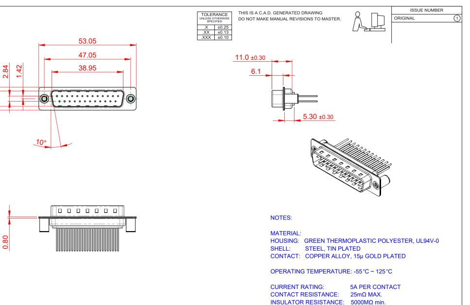
DIELECTRIC WITHSTANDING VOLTAGE: 1000V AC rms
