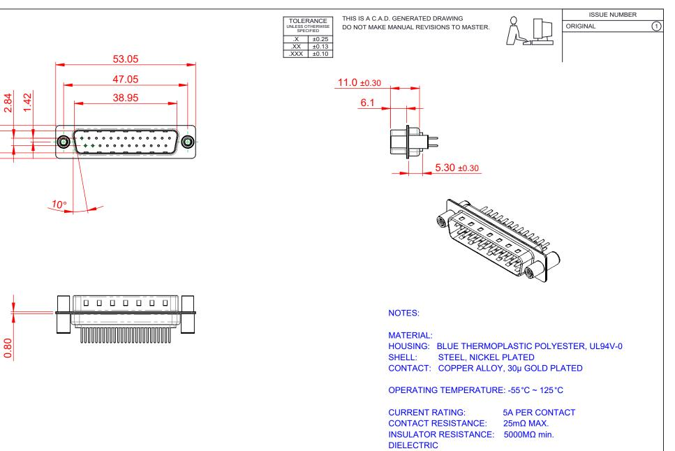
WITHSTANDING VOLTAGE: 1000V AC rms
