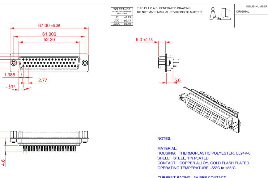
CURRENT RATING: 3A PER CONTACT CONTACT RESISTANCE: 25mΩ MAX. INSULATOR RESISTANCE: 5000MΩ min. DIELECTRIC WITHSTANDING VOLTAGE: 1000V AC rms (1)
