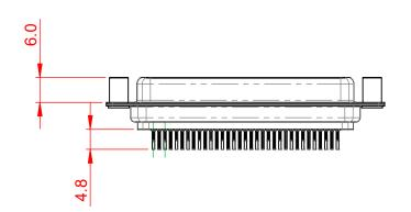
THIS IS A C.A.D. GENERATED DRAWING TOLERANCE UNLESS OTHERWISE SPECIFIED DO NOT MAKE MANUAL REVISIONS TO MASTER. .X ±0.25 .XX ±0.13
