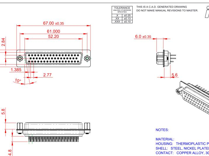
HOUSING: THERMOPLASTIC POLYESTER, UL94V-0 SHELL: STEEL, NICKEL PLATED CONTACT: COPPER ALLOY, 30µ GOLD PLATED OPERATING TEMPERATURE: -55°C to +85°C
