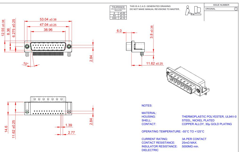
WITHSTANDING VOLTAGE: 1000V AC rms
