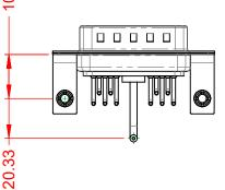
10A (CURRENT) POWER/CO-AX CONTACT RATING: (IF PRESENT) SIGNAL CONTACT CURRENT RATING: 5A PER CONTACT SIGNAL CONTACT RESISTANCE:  $10m\Omega$  MAX.
