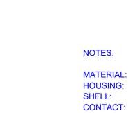
THERMOPLASTIC POLYESTER, UL94V-0 STEEL, NICKEL PLATED COPPER ALLOY, 30µ" GOLD PLATED -55°C ~ 125°C
