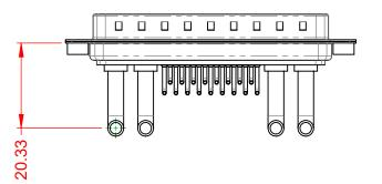
40A (CURRENT) POWER/CO-AX CONTACT RATING: (IF PRESENT) SIGNAL CONTACT CURRENT RATING: 5A PER CONTACT SIGNAL CONTACT RESISTANCE:  $10m\Omega$  MAX. **INSULATOR RESISTANCE:** 5000MΩ min. DIELECTRIC
