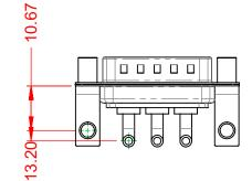
20A (CURRENT) POWER/CO-AX CONTACT RATING: (IF PRESENT) SIGNAL CONTACT CURRENT RATING: 5A PER CONTACT SIGNAL CONTACT RESISTANCE:  $10m\Omega$  MAX. **INSULATOR RESISTANCE:**
