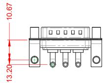
20A (CURRENT) POWER/CO-AX CONTACT RATING: (IF PRESENT) SIGNAL CONTACT CURRENT RATING: 5A PER CONTACT SIGNAL CONTACT RESISTANCE:  $10m\Omega$  MAX.
