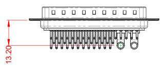
40A (CURRENT) POWER/CO-AX CONTACT RATING: (IF PRESENT) SIGNAL CONTACT CURRENT RATING: 5A PER CONTACT SIGNAL CONTACT RESISTANCE:  $10m\Omega$  MAX. INSULATOR RESISTANCE: 5000MΩ min. DIELECTRIC
