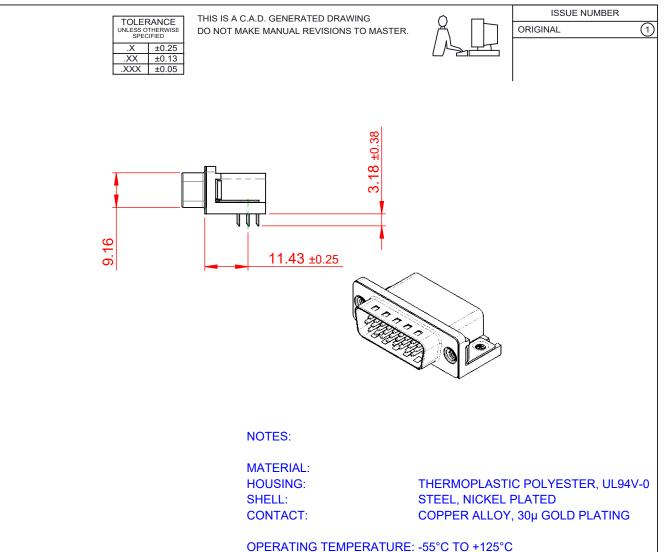
**CURRENT RATING: 3A PER CONTACT** CONTACT RESISTANCE:.  $25m\Omega$  MAX. **INSULATOR RESISTANCE:** 5000MΩ min. DIELECTRIC WITHSTANDING VOLTAGE: 1000V AC rms
