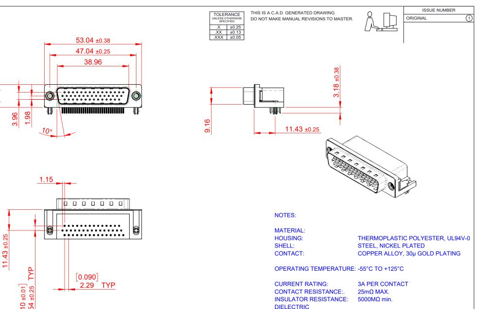
WITHSTANDING VOLTAGE: 1000V AC rms
