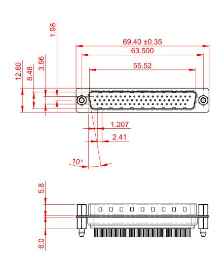
THIS IS A C.A.D. GENERATED DRAWING TOLERANCE UNLESS OTHERWISE SPECIFIED DO NOT MAKE MANUAL REVISIONS TO MASTER. .X ±0.25 .XX ±0.13
