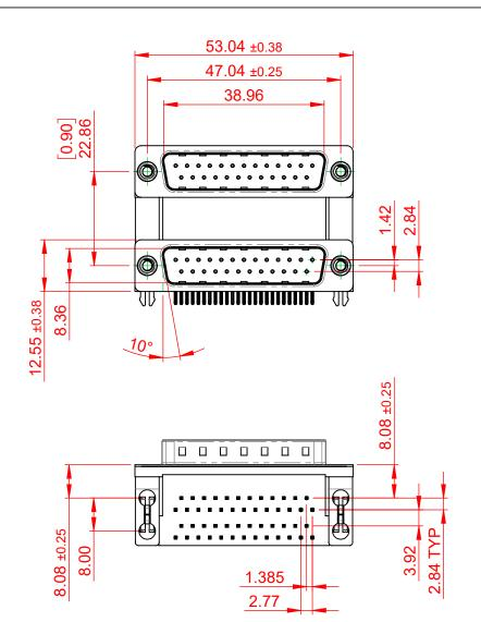
THIS IS A C.A.D. GENERATED DRAWING TOLERANCE UNLESS OTHERWISE SPECIFIED DO NOT MAKE MANUAL REVISIONS TO MASTER. .X ±0.25 .XX ±0.13
