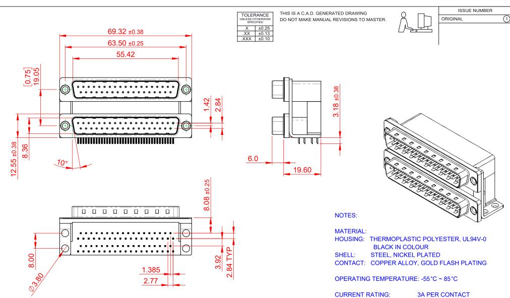
$25m\Omega$  MAX. CONTACT RESISTANCE: INSULATOR RESISTANCE: 5000MΩ min. DIELECTRIC WITHSTANDING VOLTAGE: 1000V AC rms
