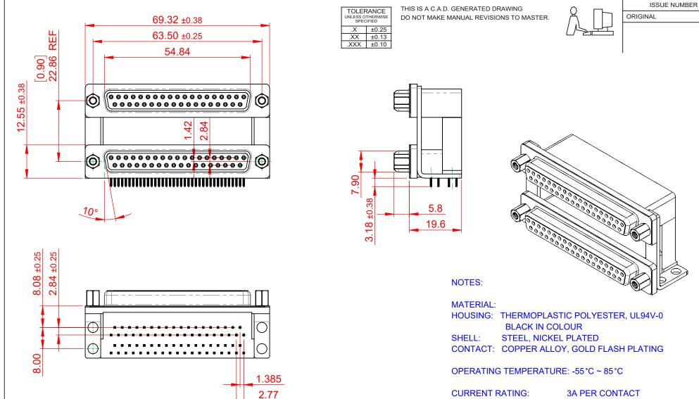
CURRENT RATING:3A PER CONTACTCONTACT RESISTANCE:25mΩ MAX.INSULATOR RESISTANCE:5000MΩ min.DIELECTRICWITHSTANDING VOLTAGE:WITHSTANDING VOLTAGE:1000V AC rms
