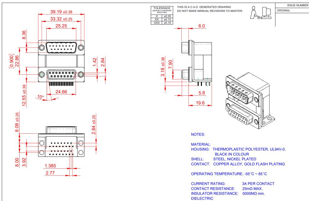
WITHSTANDING VOLTAGE: 1000V AC rms
