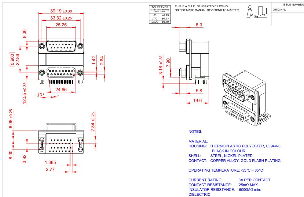
WITHSTANDING VOLTAGE: 1000V AC rms
