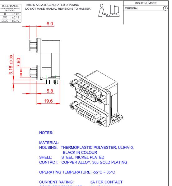
CONTACT RESISTANCE: 25mΩ MAX. INSULATOR RESISTANCE: 5000MΩ min. DIELECTRIC WITHSTANDING VOLTAGE: 1000V AC rms
