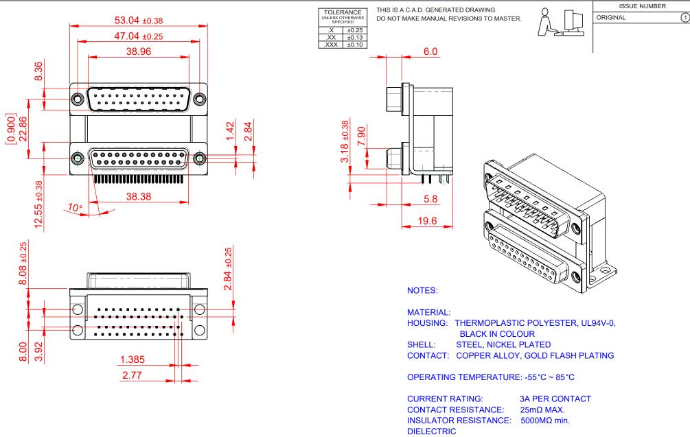
WITHSTANDING VOLTAGE: 1000V AC rms
