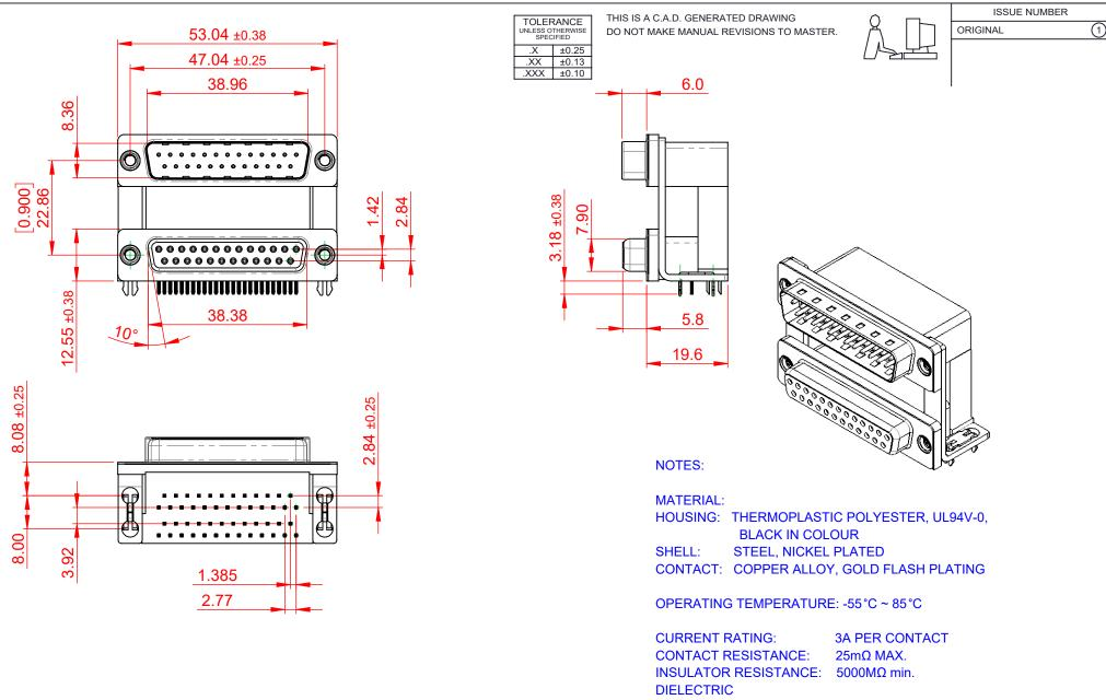
WITHSTANDING VOLTAGE: 1000V AC rms
