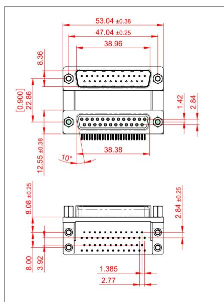
**ISSUE NUMBER** THIS IS A C.A.D. GENERATED DRAWING TOLERANCE UNLESS OTHERWISE SPECIFIED ORIGINAL (1)DO NOT MAKE MANUAL REVISIONS TO MASTER. .X ±0.25 .XX ±0.13 .XXX ±0.10 6.0 **3.18** ±0.38 6 İΤ TU 5.8 19.6 NOTES: MATERIAL: HOUSING: THERMOPLASTIC POLYESTER, UL94V-0, **BLACK IN COLOUR** SHELL: STEEL, NICKEL PLATED CONTACT: COPPER ALLOY, 30µ GOLD PLATING OPERATING TEMPERATURE: -55°C ~ 85°C
