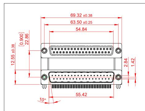
THIS IS A C.A.D. GENERATED DRAWING TOLERANCE UNLESS OTHERWISE SPECIFIED DO NOT MAKE MANUAL REVISIONS TO MASTER. .X ±0.25 .XX ±0.13 .XXX ±0.10 6 5.8 U 6.0 **3.18** ±0.38 19.6
