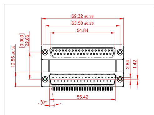
THIS IS A C.A.D. GENERATED DRAWING TOLERANCE UNLESS OTHERWISE SPECIFIED DO NOT MAKE MANUAL REVISIONS TO MASTER. .X ±0.25 .XX ±0.13 .XXX ±0.10 6 5.8 6.0 **3.18**±0.38 19.6
