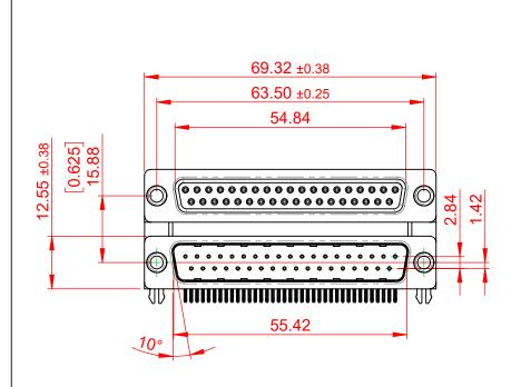
THIS IS A C.A.D. GENERATED DRAWING TOLERANCE UNLESS OTHERWISE SPECIFIED DO NOT MAKE MANUAL REVISIONS TO MASTER. .X ±0.25 .XX ±0.13 .XXX ±0.10 6 5.8
