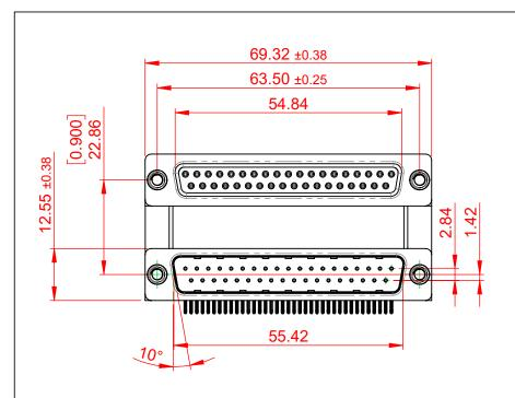
THIS IS A C.A.D. GENERATED DRAWING TOLERANCE UNLESS OTHERWISE SPECIFIED DO NOT MAKE MANUAL REVISIONS TO MASTER. .X ±0.25 .XX ±0.13 .XXX ±0.10 6 5.8 6.0 **3.18** ±0.38 19.6
