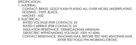
3- RECOMMENDED SOLDERING PROCESS ARE SELECTIVE SOLDERING OR MANUAL SOLDERING. OTHER FORMS OF SOLDERING SUCH AS WAVE SOLDER OR REFLOW SOLDER ARE NOT RECOMMENDED AND CAN POTENTIALLY CAUSE DEMAGNETIZATION OF MAGNET IN THE CONNECTOR
