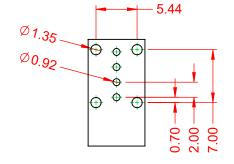
RECOMMENDED P.C.B HOLE LAYOUT TOP VIEW (TOLERANCE:±0.10)
