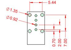
RECOMMENDED P.C.B HOLE LAYOUT TOP VIEW (TOLERANCE:±0.10)
