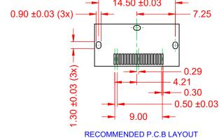
**TOP VIEW** TOLERANCE: ±1.60mm
