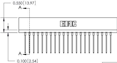
717 Series Ultra-Mate Card Edge Connector - Press Fit ACAD REFERENCE NO. 717 Part Number: 717-021-541-101
