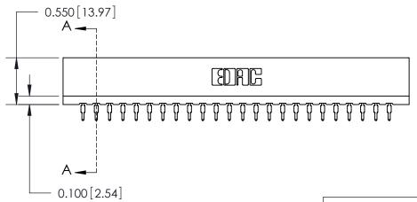
0.420 [10.67] Card Slot 0.34[8.53] 0.31 7.77 Point of Contact 0.550 [13.97] 0.300 [7.62] SECTION A-A
