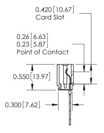
Note: MBB switching contacts assembled in specified positions are available on request. 717 Series Ultra-Mate Card Edge Connector - Press Fit
