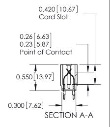
717 Series Ultra-Mate Card Edge Connector - Press Fit
