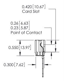
717 Series Ultra-Mate Card Edge Connector - Press Fit
