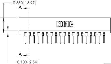
717 Series Ultra-Mate Card Edge Connector - Press Fit ACAD REFERENCE NO. Part Number: 717-038-522-201
