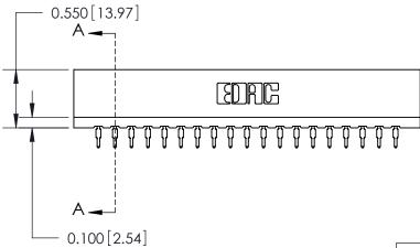
717 Series Ultra-Mate Card Edge Connector - Press Fit Part Number: 717-038-525-201
