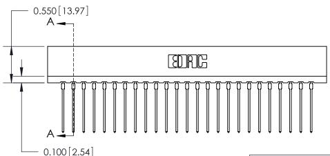
717 Series Ultra-Mate Card Edge Connector - Press Fit
