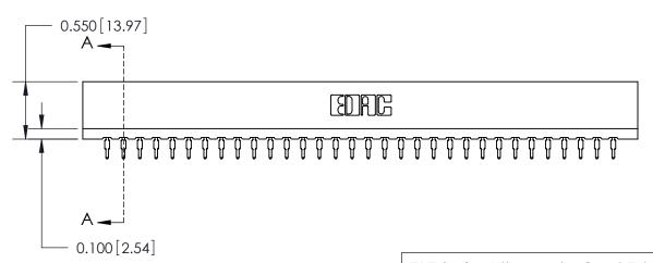
0.420 [10.67] Card Slot 0.34[8.53] 0.31 7.77 Point of Contact 0.550 13.97 0.300 [7.62] SECTION A-A
