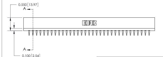
Note: MBB switching contacts assembled in specified positions are available on request. 717 Series Ultra-Mate Card Edge Connector - Press Fit ACAD REFERENCE NO. 717-ENG MASTER Part Number: 717-066-560-206
