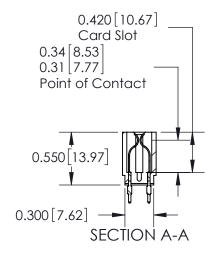
Note: MBB switching contacts assembled in specified positions are available on request. 717 Series Ultra-Mate Card Edge Connector - Press Fit Part Number: 717-068-525-206
