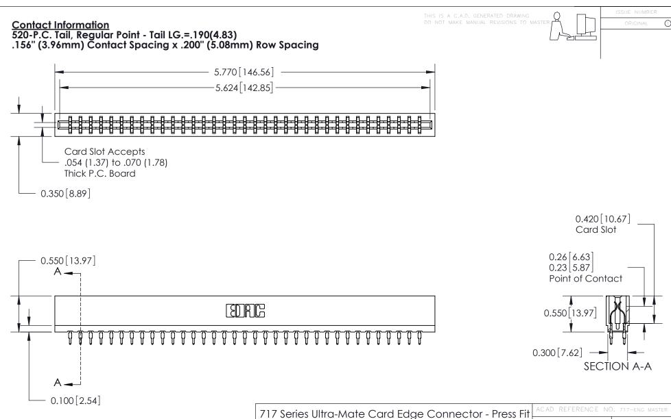
Note: MBB switching contacts assembled in specified positions are available on request. Part Number: 717-070-520-206
