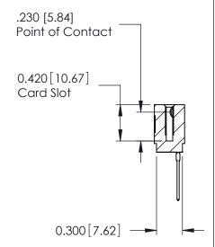
ACAD REFERENCE NO. 725-ENG MASTER 725 Series Ultra-Mate Card Edge Connector - Press Fit SEGAHOM:3A:9A DRAWN: J.LEE Part Number: 725-005-545-101 CHECKED: DATE: **EDAC INC** SCALE: SHEET 1 OF 1 THESE DRAWINGS AND SPECIFICATIONS ARE THE PROPERTY OF EDAC INC.,AND TORONTO, ONTARIO SHALL NOT BE REPRODUCED, OR COPIED DRAWING NUMBER **ISSUE** CANADA OR USED AS THE BASIS FOR THE 725-ENG MASTER MANUFACTURE OR SALE OF APPARATUS YOUR CONNECTION TO QUALITY & SERVICE WITHOUT WRITTEN PERMISSION.
