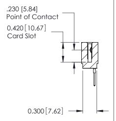
ACAD REFERENCE NO ECTION SARA 725 Series Ultra-Mate Card Edge Connector - Press Fit DRAWN: Part Number: 725-007-522-101 CHECKED: **EDAC INC** THESE DRAWINGS AND SPECIFICATIONS ARE THE PROPERTY OF EDAC INC.,AND TORONTO, ONTARIO SHALL NOT BE REPRODUCED, OR COPIED CANADA OR USED AS THE BASIS FOR THE MANUFACTURE OR SALE OF APPARATUS YOUR CONNECTION TO QUALITY & SERVICE
