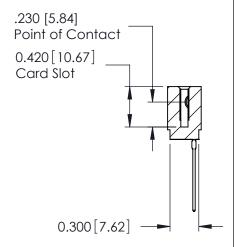
ACAD REFERENCE NO. 725-ENG MASTER 725 Series Ultra-Mate Card Edge Connector - Press Fit DRAWN: DATE: AUG31/09 J.LEE Part Number: 725-010-541-101 SEGTION A-A CHECKED: SHEET 1 OF 1 **EDAC INC** SCALE: THESE DRAWINGS AND SPECIFICATIONS ARE THE PROPERTY OF EDAC INC.,AND TORONTO, ONTARIO SHALL NOT BE REPRODUCED, OR COPIED DRAWING NUMBER **ISSUE** CANADA OR USED AS THE BASIS FOR THE 725-ENG MASTER MANUFACTURE OR SALE OF APPARATUS YOUR CONNECTION TO QUALITY & SERVICE WITHOUT WRITTEN PERMISSION.
